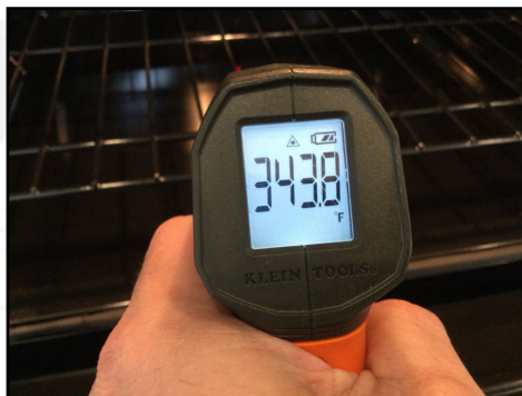
Temperature measured inside oven when set to 350 degrees
