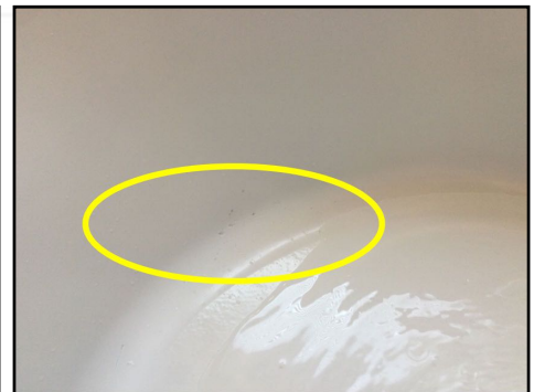
Gouged observed along interior primary tub
